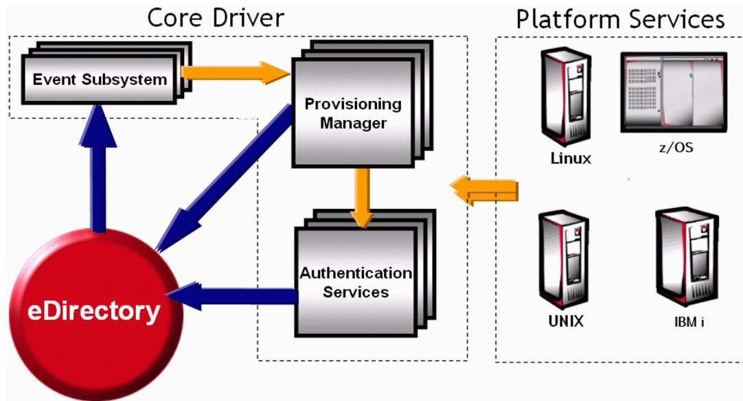
The Core Driver provides Authentication Services and information about changes to users and groups to target platforms that have been configured to run Platform Services.
