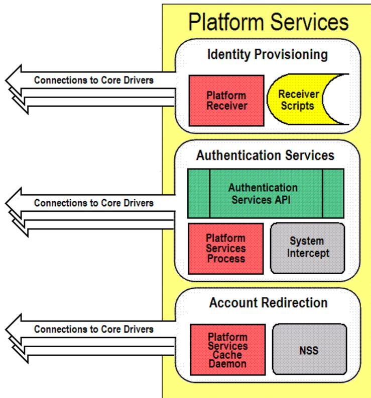
The Platform Services System Intercept is hooked into the login process of a system using standard, vendor-provided mechanisms. It provides password verification and password change functions.
