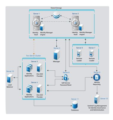
You can easily add additional identity applications and OSP servers (or nodes) to handle the load, then add new servers to the L4 switch. When the new servers are added to the cluster, they are automatically sent the cluster configuration.
