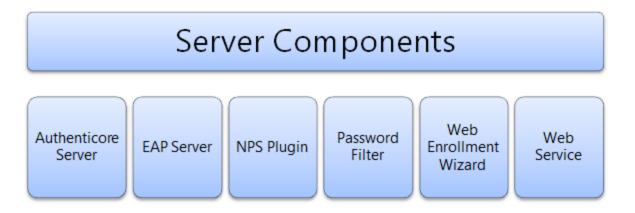
**Authenticore Server** is the central component in an NetlQ Advanced Authentication Framework Enterprise deployment. It is intended for processing NetlQ Advanced Authentication Framework users authentication requests. Information about it is represented in the following guides:
