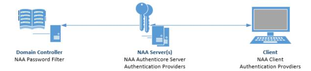
NetIQ Password Filter is installed on the Domain Controller.
