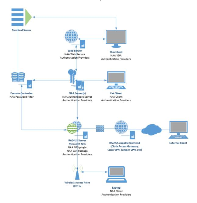
NetIQ Password Filter is installed on the Domain Controller.
