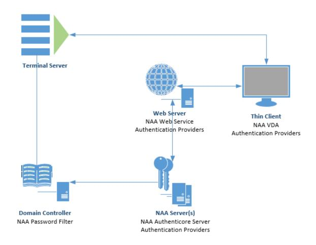
NetIQ Password Filter is installed on the Domain Controller.
