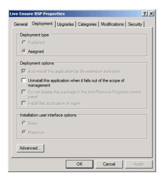
b) On the **Deployment** tab: click the **Advanced** button and select the **Ignore language when deploying this package** check box. If you do not select this check box, the package will be installed only on OS with package's language.
