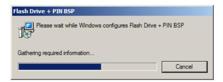
The start of installation may be frozen for a time up to 1 minute in the case of offline mode. This delay occurs due to check of digital signature of component.
