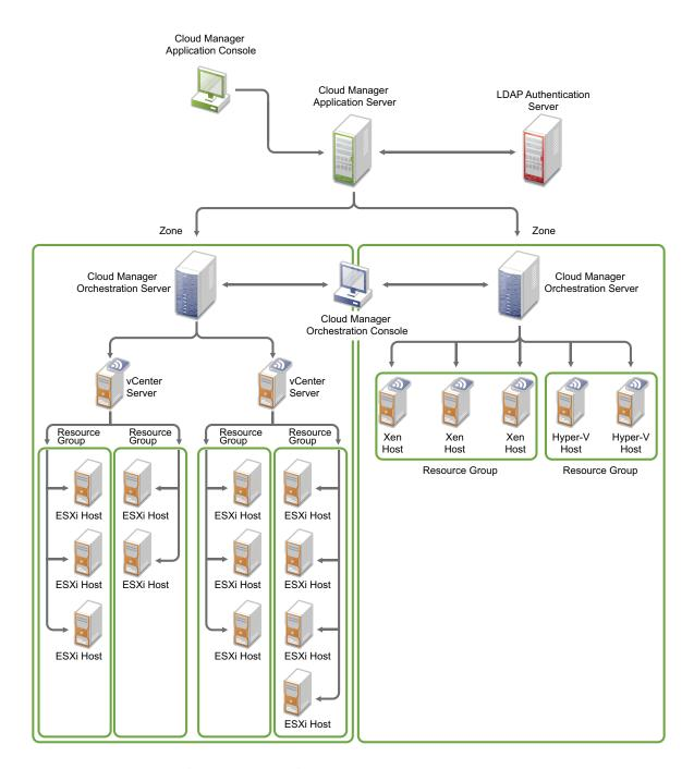
A resource group identifies a collection of hosts (and their associated networks and storage). When a workload is deployed, it is assigned to the resource group and provisioned using any of the resources within the group.
